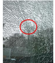
breakages. Heat soaked toughened glass is 95% more susceptible to failure due to nickel sulphide inclusion during the manufacturing process rather than later on site. The additional cost per unit ranges for this process is on average from 7% to 10% extra.
