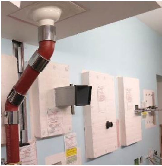
Figure 31 A sample of a penetration seal system
