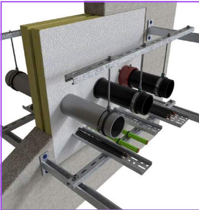
Figure 21 Multiple services within a single opening
