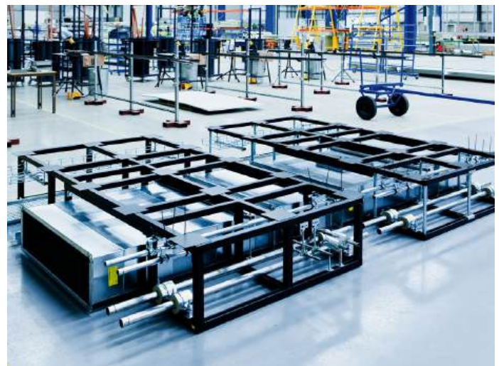
Figure 4 Example of a prefabricated corridor M&E module
