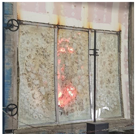
Figures 7 Glazed partition in a supporting construction during testing, where the intumescent interlayer has reacted to provide thermal insulation
